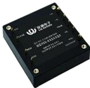
◆宽范围输入Wide Input voltage range (2:1) ◆转换效率典型90%，Typical Efficiency 90% ◆开关频率 Switching frequency：300 KHz ◆过流、短路保护，自动恢复 Over current/Short circuit protection, Self-furbish ◆输入与输出高隔离 Input-output isolate (1500Vdc) ◆PCB板上直插式安装 PCB Board in-line type installs ◆铝基板Aluminum baseplate, 输出波纹低 Low Output Ripple ◆高功率密度 High power density 详情请访问我们的网站：<http://www.aipu-elec.com>
